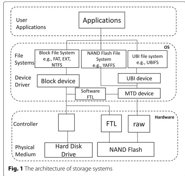
**Fig. 1** The architecture of storage systems
