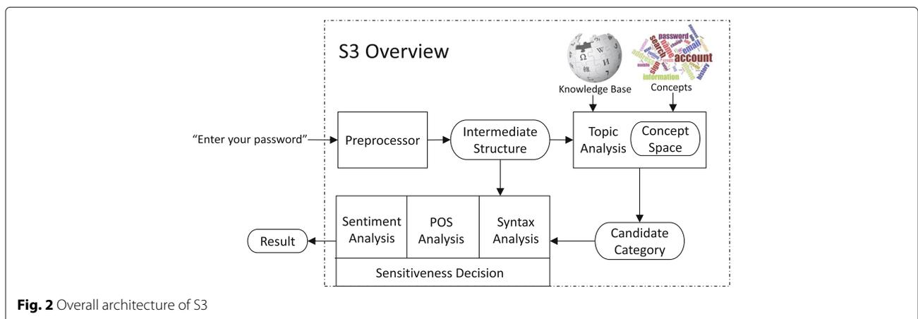
**Fig. 2** Overall architecture of S3
