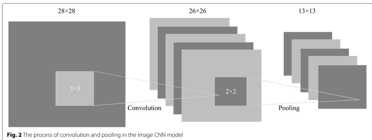
**Fig. 2** The process of convolution and pooling in the image CNN model
