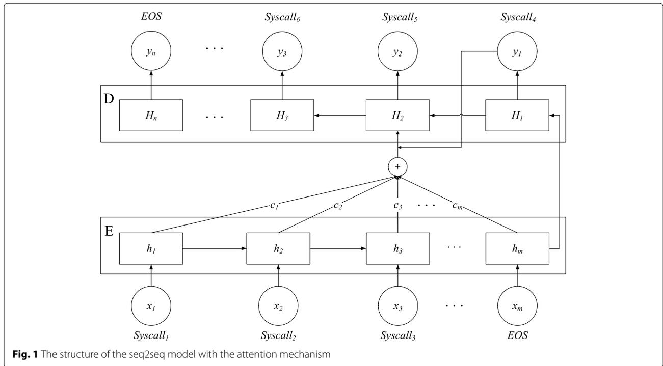
**Fig. 1** The structure of the seq2seq model with the attention mechanism
