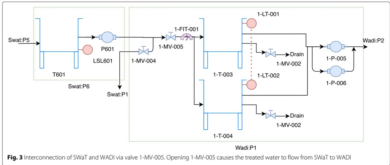
to OPEN, 1\_MV\_005 to CLOSE, and pump P601 is turned OFF. SWaT and WADI are clearly interdependent based on condition 1 (as discussed in “Interdependency among critical infrastructure” section), i.e. input of one system is the output of the other.
