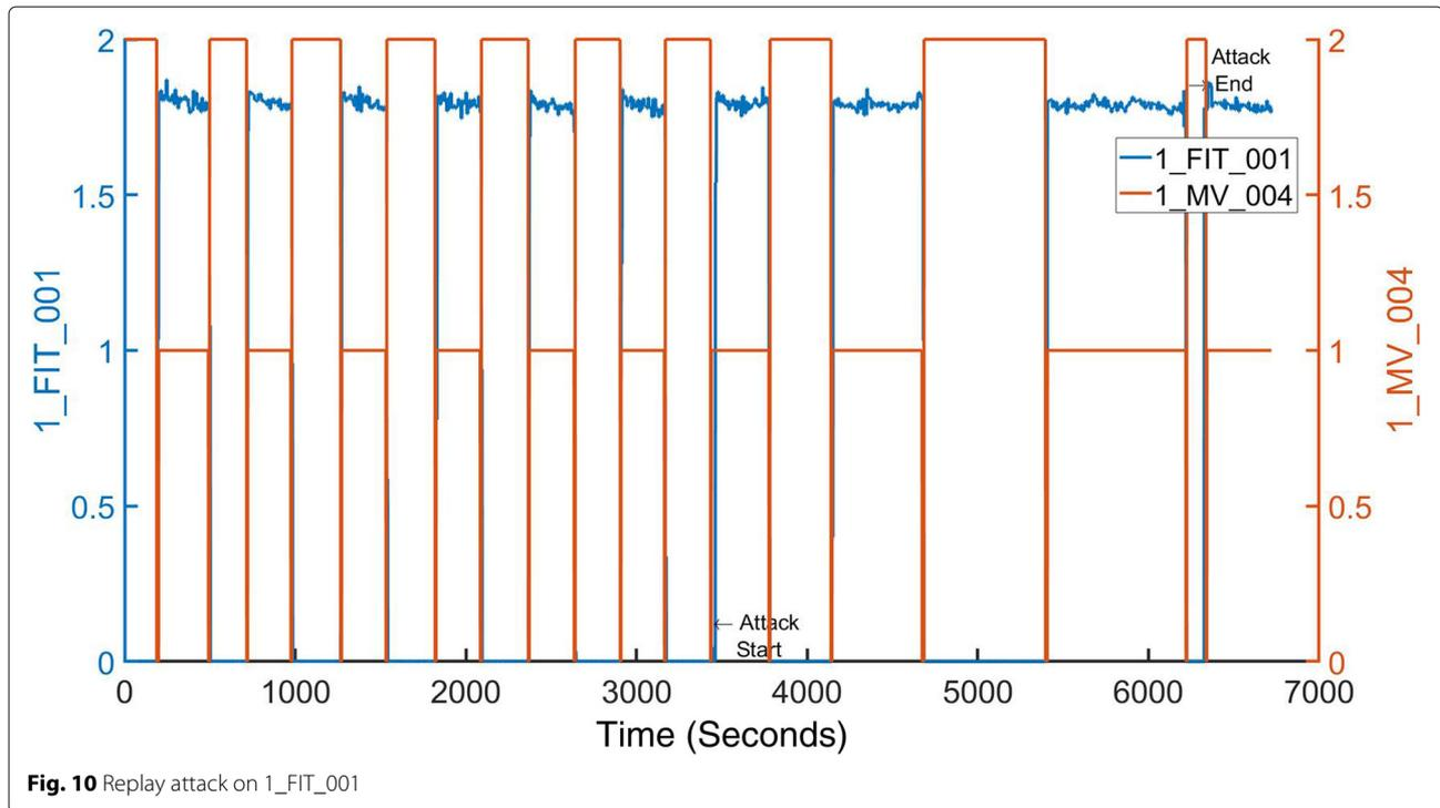
Fig. 10 Replay attack on 1\_FIT\_001
