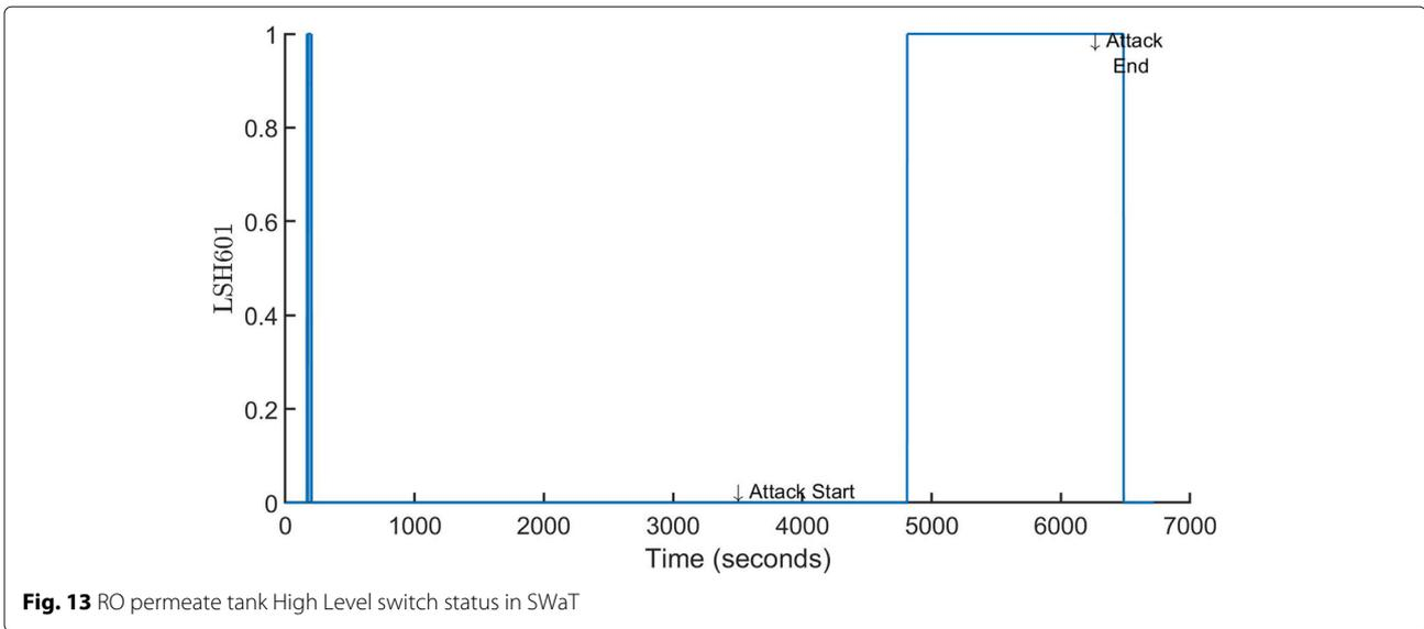
Fig. 13 RO permeate tank High Level switch status in SWaT
