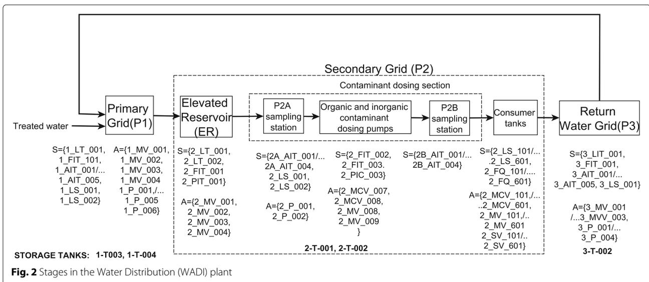
**Fig. 2** Stages in the Water Distribution (WADI) plant
