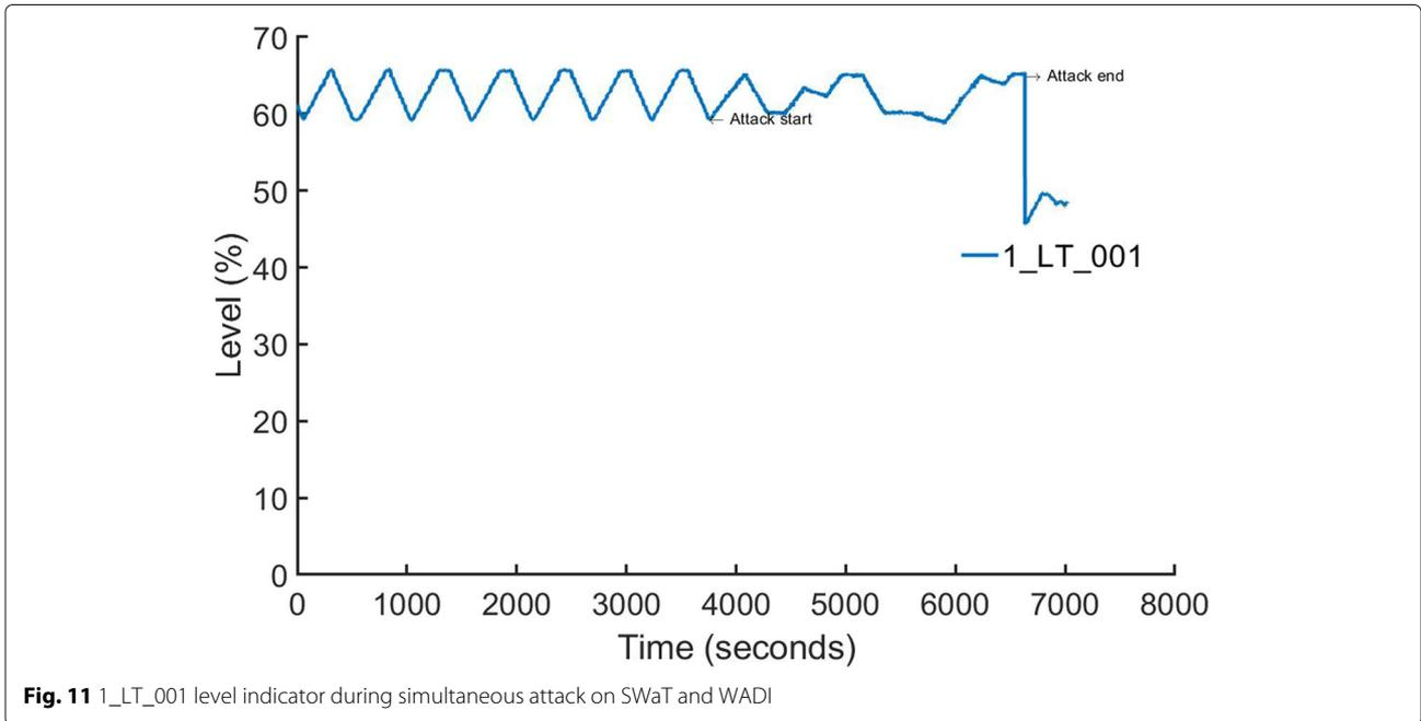
second ( $AS_{1A_3}$ ) mark. Consequently the PLC assumes that the water quality is not within the acceptable range. This leads to the opening of valves 1\_MV\_002 and 1\_MV\_003 to drain the water in the raw water tank. When the level reaches the Low mark, water from the RO tank will be supplied. Due to this attack, water supply from the RO
