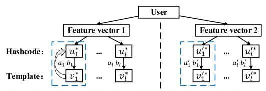
Fig. 10 An explanation of ARM attack to our proposed scheme. The two sides of the black dotted line represent the template generations by same distance-preserving hashing of feature vectors of the same user with different tokens
