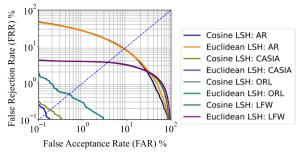
Fig. 9 ROC curves of our scheme over various databases under stolen-token scenario
