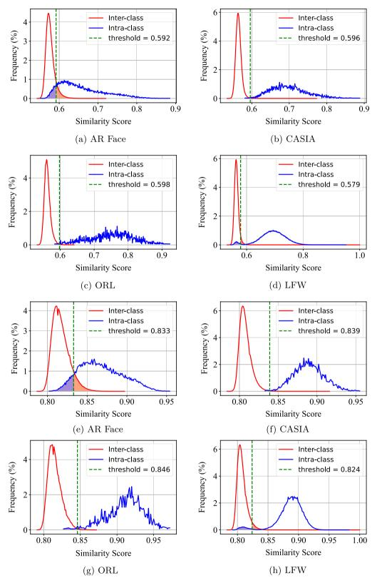
**Fig. 4** Threshold of schemes with Euclidean LSH under k = 5000, n = 2, c = 1.0 and Cosine LSH under k = 10,000, N = 2, d = 2. **a**–**d** show the result of Euclidean LSH-based scheme, while **e**–**h** show the result of Cosine LSH-based scheme
