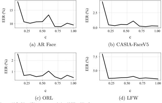
**Fig. 5** EER change with Euclidean LSH parameter *c* under k = 10,000 and N = 2
