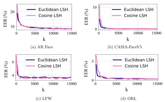
**Fig. 7** EER changes with LSH length k under c = 1.0, d = 2 and N = 2
