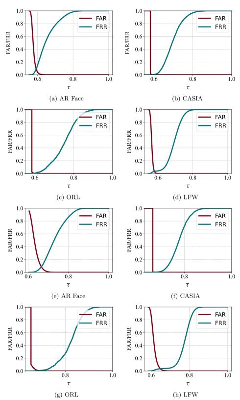
**Fig. 8** FAR and FRR change with threshold  $\tau$  for Euclidean LSH under k = 5000, N = 2, c = 1.0 and Cosine LSH under k = 10,000, N = 2, d = 2. **a**–**d** show the result of Euclidean LSH-based scheme, while **e**–**h** show the result of Cosine LSH-based scheme
